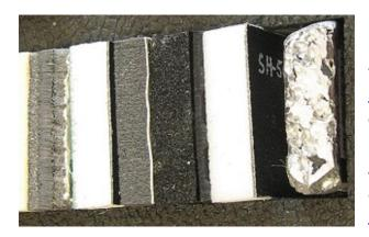
Heat management materials include melamine and polyimide foams, aluminum foil-faced fiberglass fabric composites, and closed-cell <u>custom thermal insulation</u> that's designed to stop the propagation of flame and smoke.
